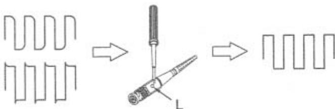
Adjust trimmer L until seeing flat-top square wave on the display.
